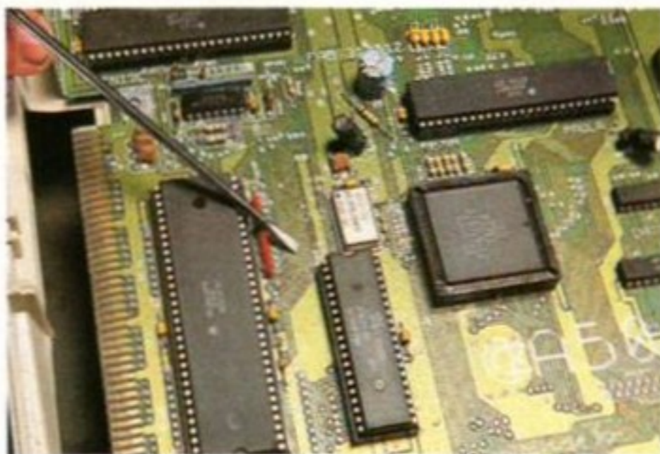
Revision 6A boards are considerably less cramped than revision 5s, so it's even easier to cut the right track and make a bridge
